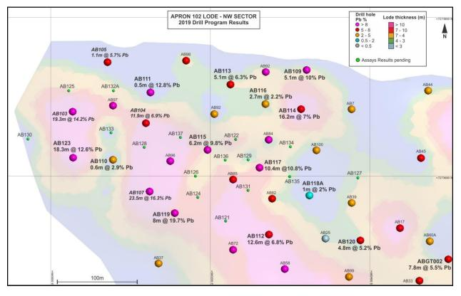
Figure 4: Plan view of the Apron Zone 102 Lode showing drillhole pierce points (coloured by lead grade) and lode thickness contours (N.B. thickness contours include visual thickness estimates from logged mineralisation for holes with pending assays)
