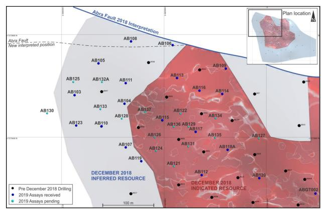
Figure3: Plan view of the northwestern area of the December 2018 Resource Apron Zone showing drill-hole pierce point positions
