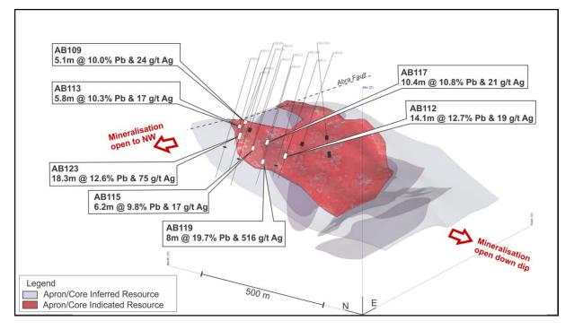
Figure 1: 3D model of December 2018 Resource (5% lead cut-off wireframes) looking obliquely east, with new drill-holes AB103 – AB120, AB123 and ABGT002 overlain
