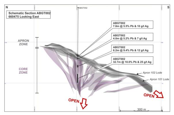
Figure 2: Schematic cross section of December 2018 Resource (5% lead cut-off wireframes) looking obliquely east, with new drill-hole ABGT002 overlain
