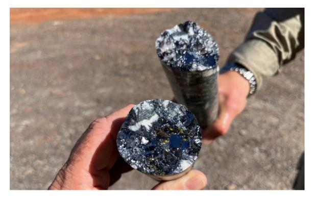
**Figure 3** – Image of some of the spectacular galena mineralisation being seen in the underground grade control and infill drilling program.
