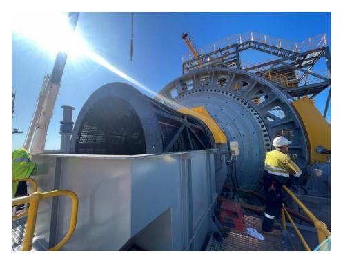
Figure 11 – Mill discharge assembly.
