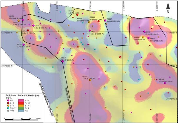
Figure 2. Plan view of Abra Apron Zone 102 lode showing drill-hole pierce point, coloured according to the lead grade range, for the historical (small points) and 2020 Abra Drilling Program drill-holes (large points), over the mineralisation domain thickness contour map.
