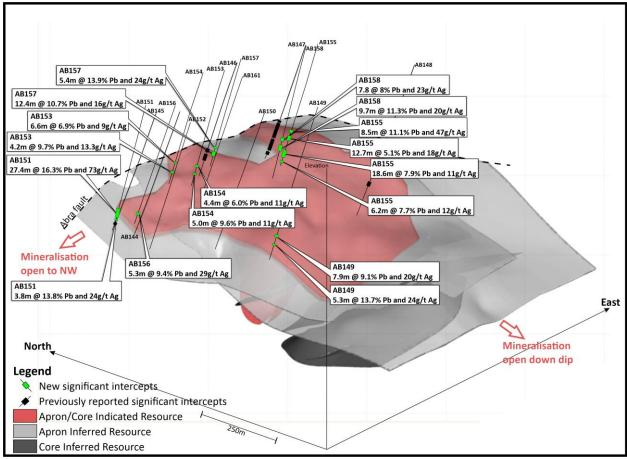
Figure 1. 3D model of October 2019 Resource (5% lead cut-off wireframes) looking obliquely northeast, with new drill-holes AB149 to AB158, showing significant mineralised intersections.
