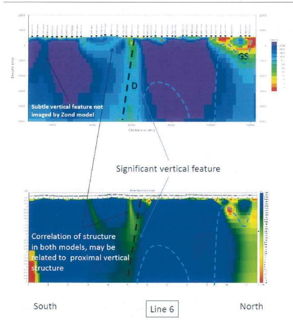
Figure 7 - Woodlands MT/AMT line showing steeply dipping deep structure
