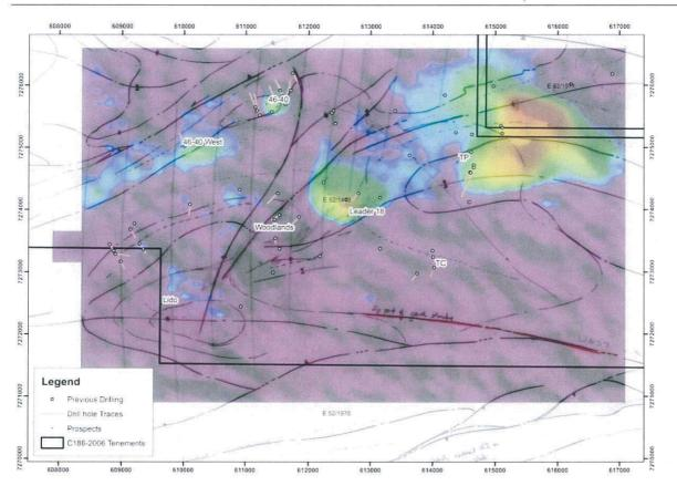
$Figure\ 6-Untested\ Late-time\ Anomaly\ at\ TP\ with\ Tested\ Anomalies\ at\ Leader\ 18\ and\ 46-40\ MT/AMT\ Survey$
