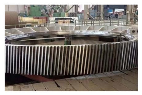
Figures 12 – New mill girth gear nearing completion.
