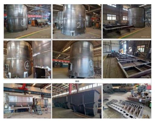
Figure 10 – Flotation cell fabrication.
