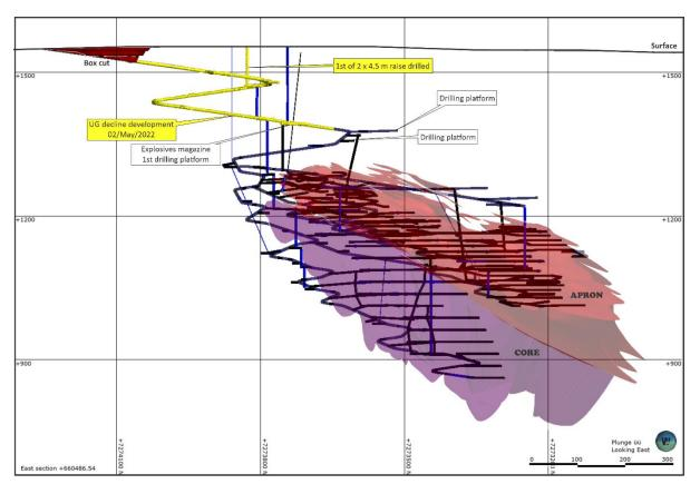
**Figure 4** - Shows the progress of the Abra underground mine development to the 2<sup>nd</sup> of May (yellow).
