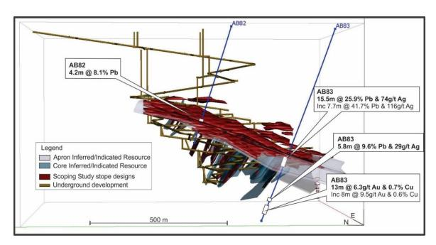
Figure 4: 3D model of the core and apron zones looking east showing AB82 and AB83, March 2018 Inferred and Indicated Resources outlines (>5% Pb wireframes) and scoping study underground mine development and stopes.
