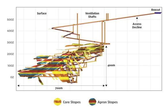
Figure 1: Abra's Conceptual Mine Design - Long Section View
