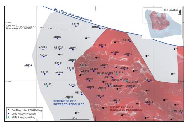
Figure 2: Plan view of the northwestern area of the December 2018 Resource Apron Zone showing drill-hole pierce point positions
