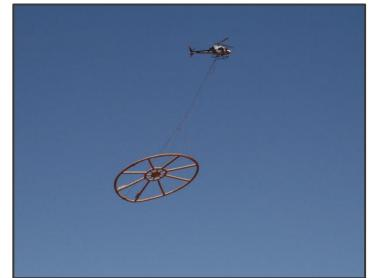
Figure 2: New Resolution Geophysics (NRG<sup>™</sup>) Australia carrying out a high-resolution helicopter hosted airborne electromagnetic (EM) survey over the Woodlands Complex
