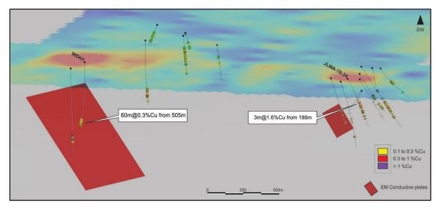
Figure 3: Woodlands 3D view looking south west of EM anomalies at surface, EM conductive plates and historic drill holes
