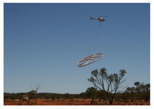
Figure 2: Helicopter-borne Electromagnetic (EM) survey underway at Woodlands
