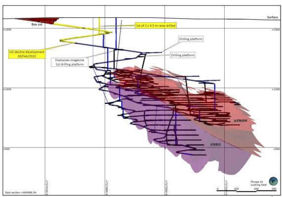
**Figure 1** – Long section showing the completed mine development location by 28<sup>th</sup> February.
