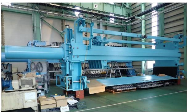
Figure 10 – Plate filter (Ishigaki) ready for shipping from Japan.
