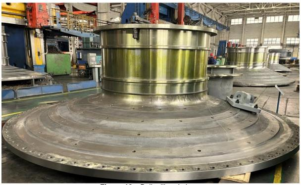
Figure 12 - Ball mill end piece.
