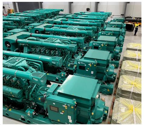
Figure 9 – Power station generation units in Perth ready for transport to site.
