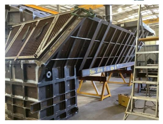
Figure 8. Primary crusher feed chute fabrication (Perth).
