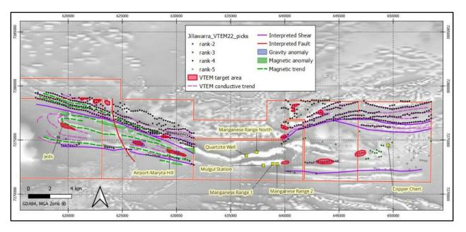
Figure 14. Jillawarra Project tenement outlined in red over the regional filtered magnetic image (total magnetic intensity, reduced to pole, 1st vertical derivative, automatic gain control) with the VTEM anomaly picks shown as coloured dots, VTEM target areas, interpreted structures, and geophysical trends. (Source: Resource Potentials – JW VTEM 2022 Memo)
