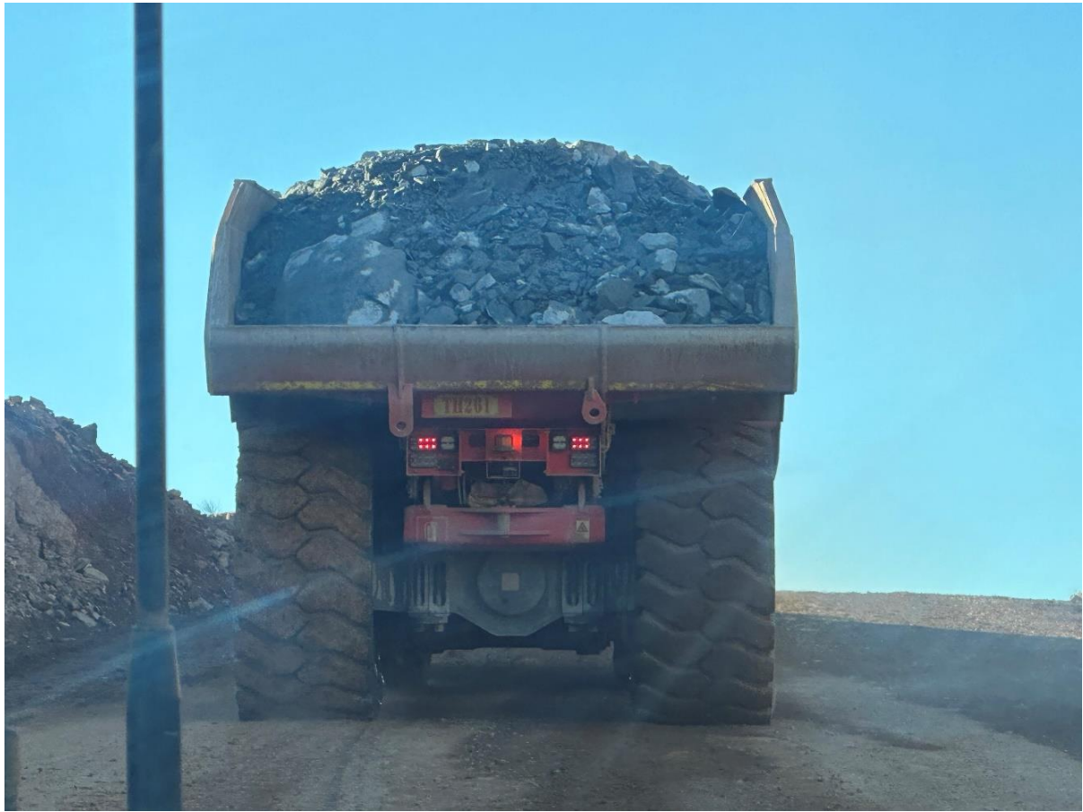
Figure 9 – Underground truck hauling ore out of Abra decline (Photo 13 July 2023).
