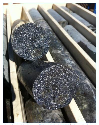
Figure 2: Massive galena (lead sulphide) from 407.5 to 409.5m in AB071 (hole ongoing) showing over 50% galena over 2 metres within a broader zone of +5% galena mineralisation over broad zones (+5 metres).
