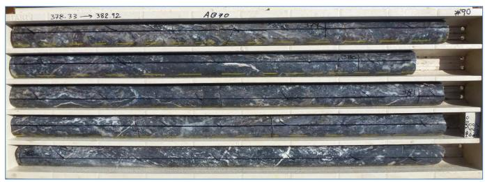
Figure 1: Example of strong galena (lead sulphide) mineralisation in hole AB070 through interval in core tray. Visual galena mineralisation is above 10% over this tray (5m intercept). This tray lies within other broad zones of galena mineralisation.
