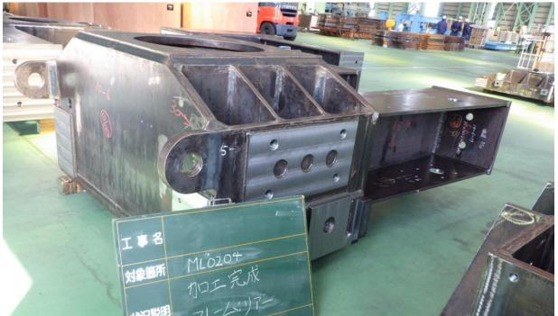
Figure 6 – Abra concentrate filter frame assembly (Ishigaki, Japan).
