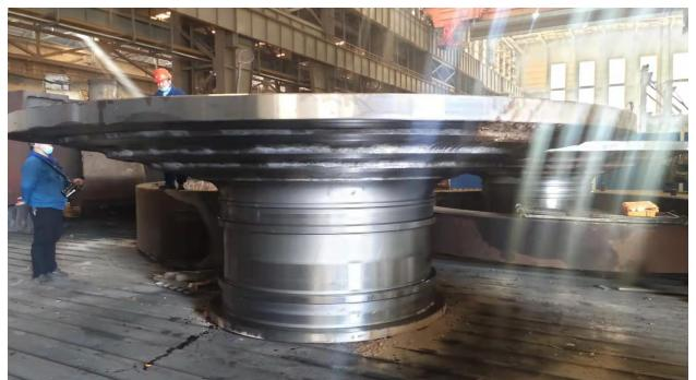
Figure 7 – Abra ball mill head end inspection (CITIC-Heavy Industries Co. Ltd., China).
