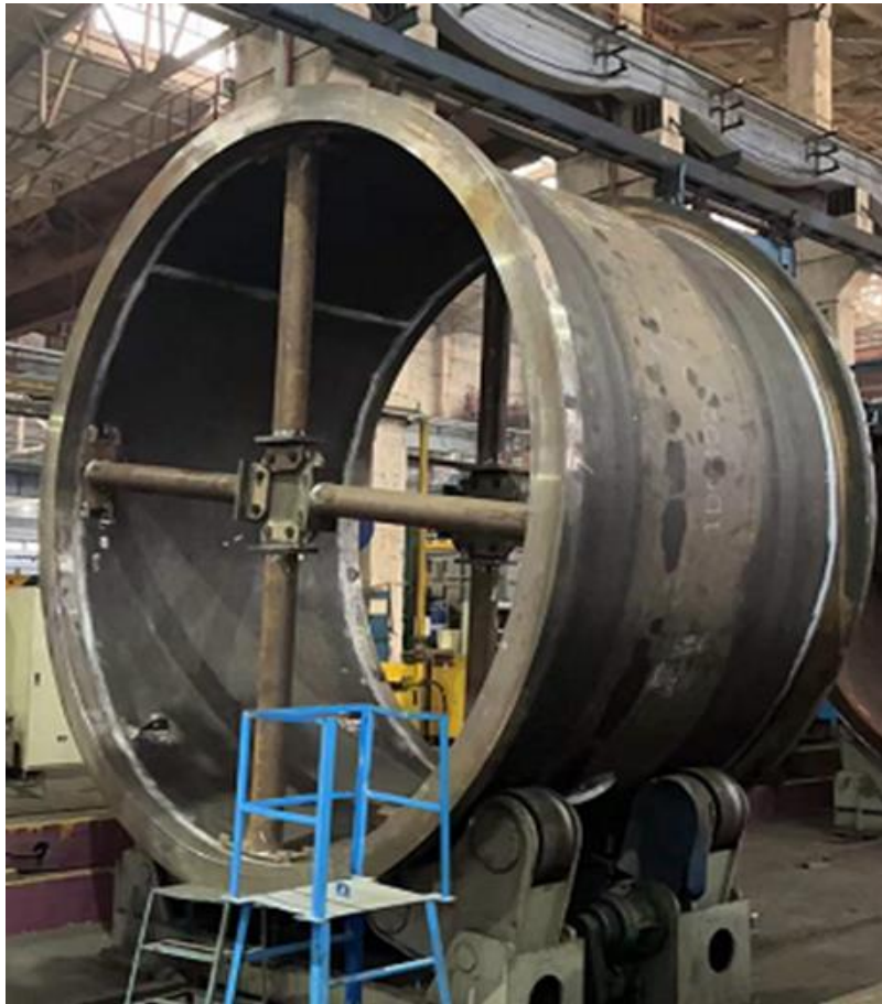
Figure 6. Processing Plant equipment fabrication (ball mill shell welding).
