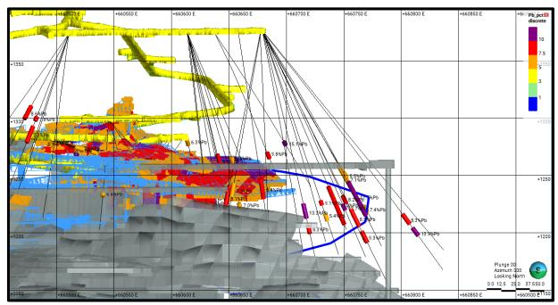
Figure 2 – Shows long section view looking north with location of some of the new drill holes on the northeastern end of the deposit that will generate new mining shapes that will be included in the mine plan moving forward. Coloured mining shapes shown in Figures 1 & 2 are the same mining shapes scheduled to be mined out to June 2024. Grey mining shapes are those currently scheduled after June 2024.
