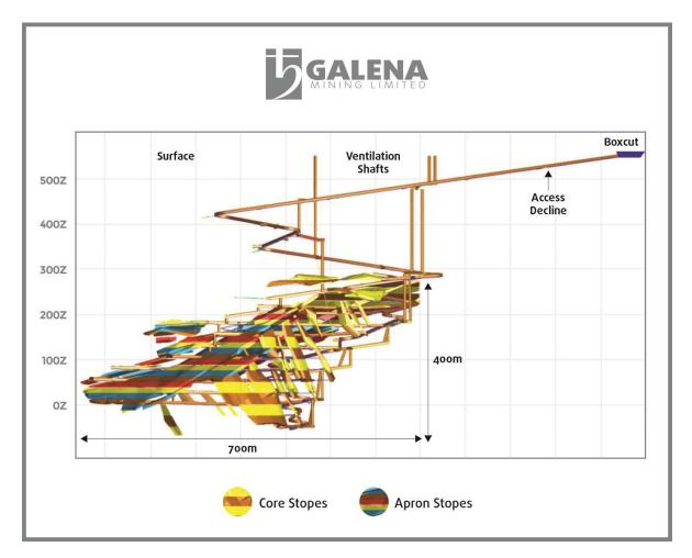
Figure 1: Abra's Conceptual Mine Design – Long Section View
