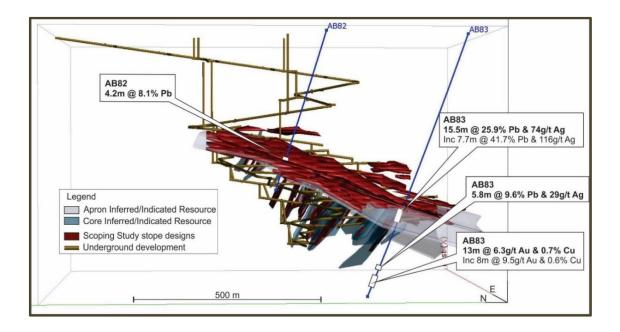
Figure 5: 3D model of the core and apron zones looking east showing AB82 and AB83, March 2018 Inferred and Indicated Resources outlines (>5% Pb wireframes) and scoping study underground mine development and stopes
