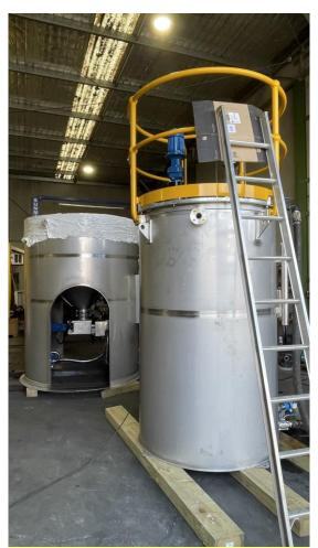
Figure 6 – Flocculant mixing plant fabrication.
