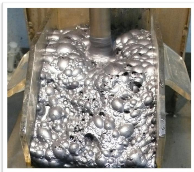
Figure 1: High-grade lead-silver concentrate taken during recent test-work on Abra samples.
